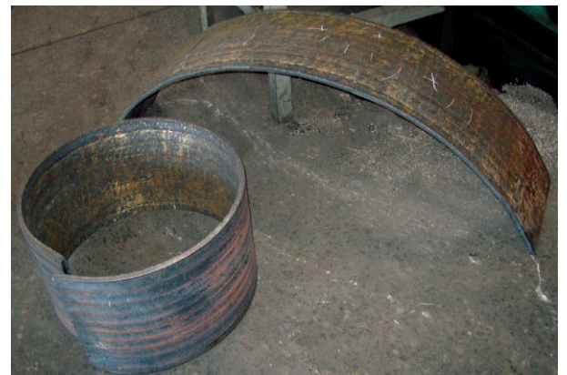
OD, top, and ID radii for a typical single pass SHS 9700 overlay.
