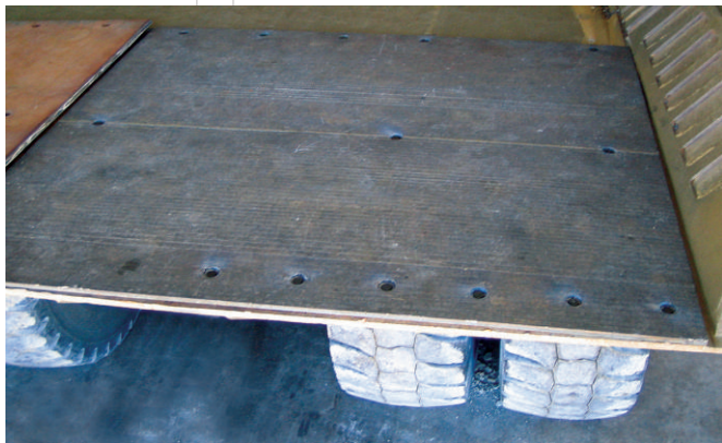
SHS 9700 wear plate (9'x8') after installation in October 2007.
