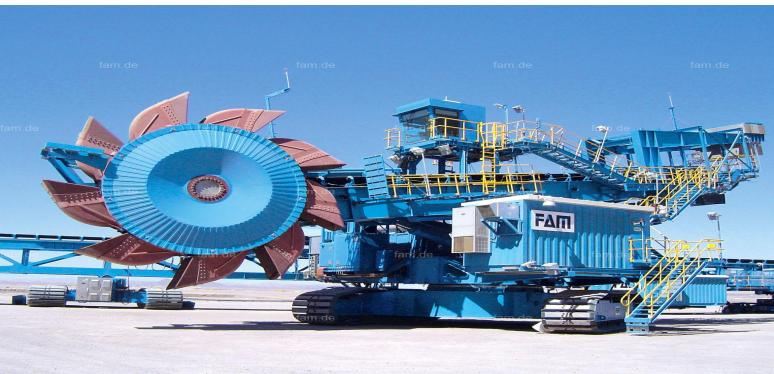
**Trench type** stacker reclaimers are ideal for installations with low-volume, high active storage pile capacities.
