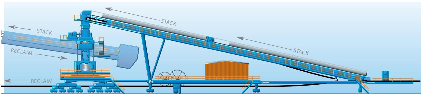
**Straight-Through Tripper** is utilized when material enters the storage yard from one end of the yard and leaves toward the other end. If facility operation is such that some or all of the material may bypass the storage yard, a splitter gate can be mounted at the tripper head chute.
