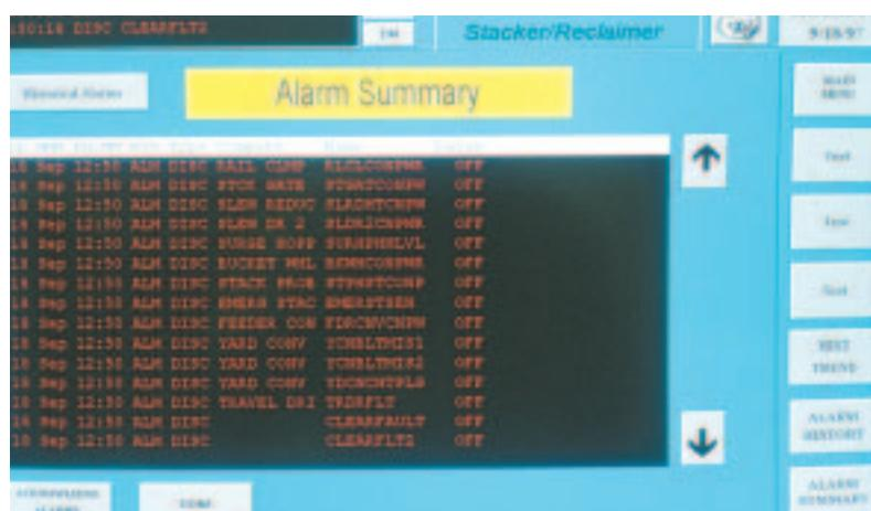
Alarm/fault diagnostic logic is included in all stacker reclaimer control systems, minimizing troubleshooting by immediately pinpointing the problem source.
