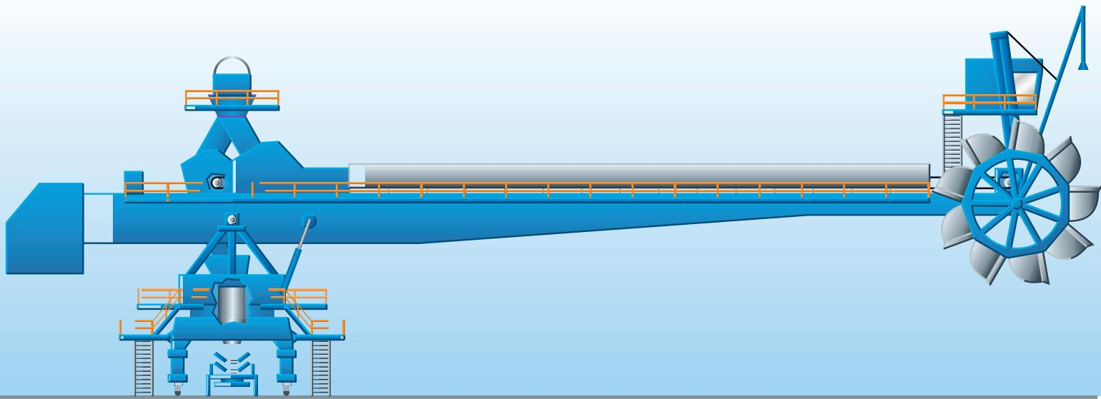
**Straight-Through Boom Configuration** provides rapid, efficient stacking and reclaiming of materials in an environment where boom length need not exceed 125 feet (38 meters). Ports, terminals, and power plants generally utilize this design when less expansive storage is required.
