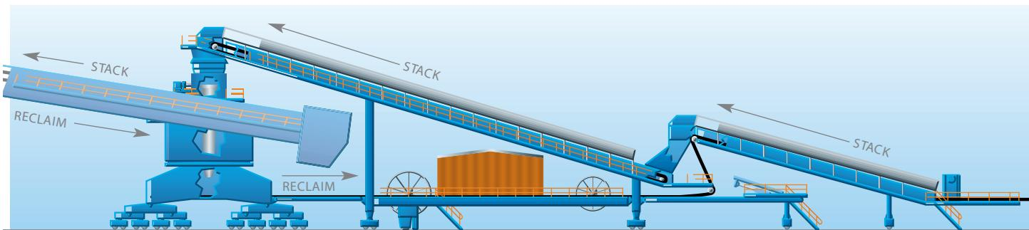
**Articulating Tripper** is used when material enters and leaves the storage area from the same end of the yard. By articulating the tripper structure, this section can be lowered (retracted) for reclaiming operation.
