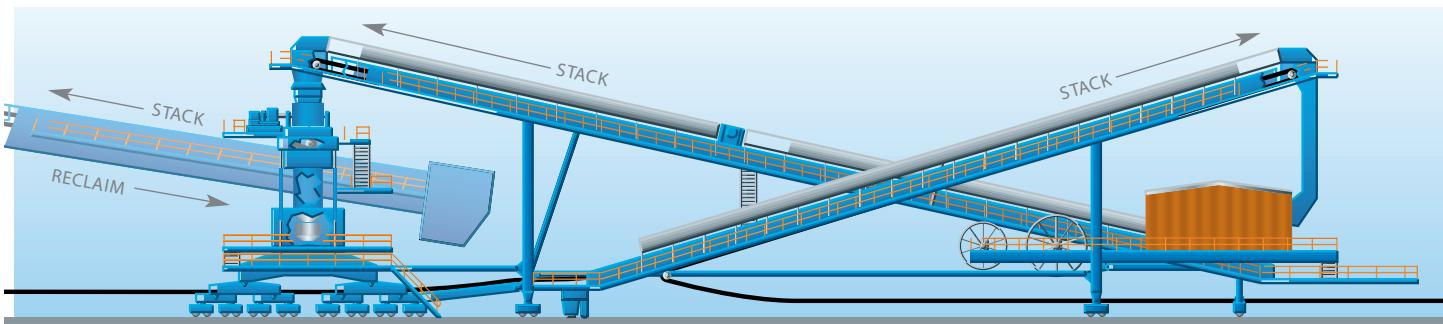
**Scissors-Type Tripper** is also used when material enters and leaves the storage area from the same end of the yard. This tripper utilizes a separate elevating conveyor to direct the material to the centerline of rotation for stacking.
