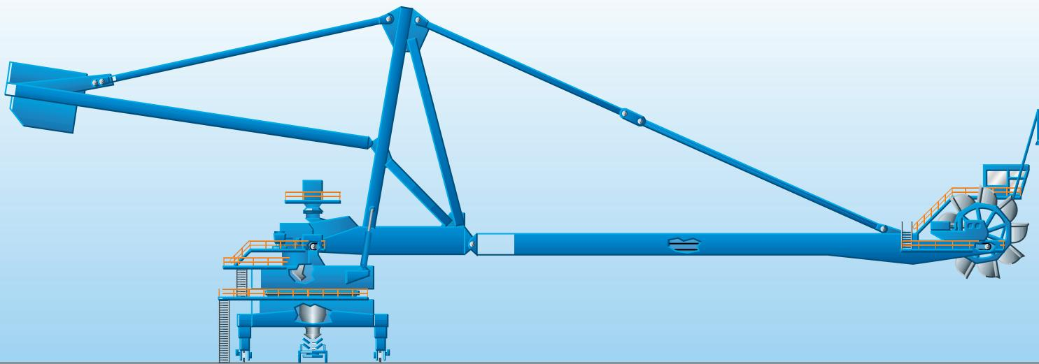
**Masted Boom Configuration** is designed for use in applications where extended boom length (over 125 feet/38 meters) is necessary. The added support reduces excessive boom flex inherent in long-reaching stacker reclaimers or where high digging forces cause unacceptable boom tip deflection.
