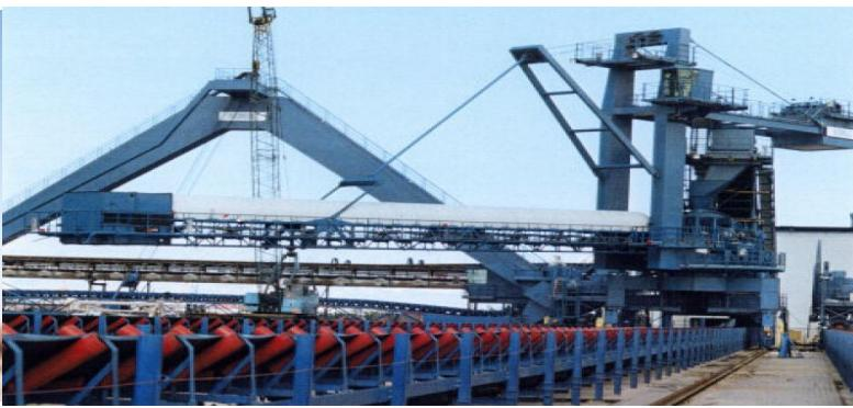
**Masted Boom** slewing type stacker reclaimers are used in facilities requiring higher live storage quantities.
