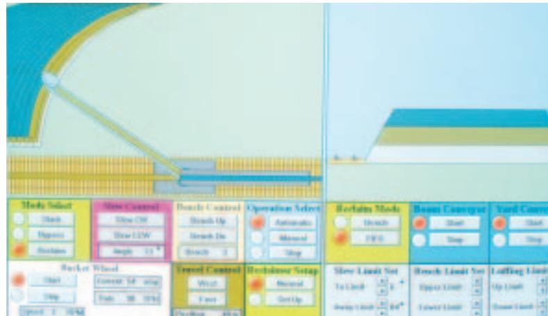
MMI system provides total intelligent operator system control. In the event of a problem, the MMI display instantly pinpoints the trouble area.
