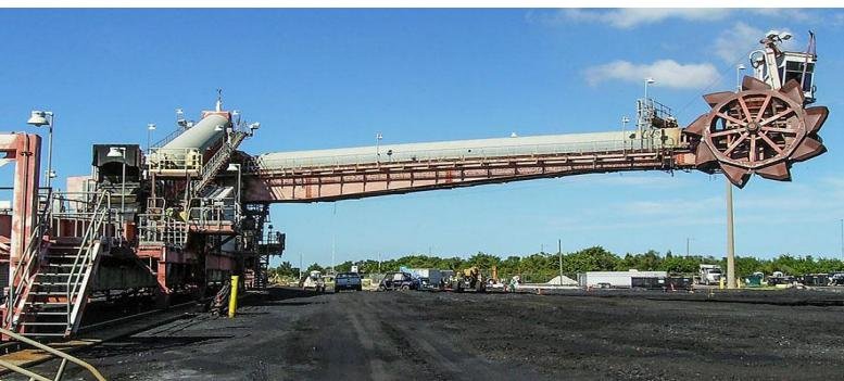
**Straight-Through Boom** slewing type machines typically are suitable for most storage facilities.
